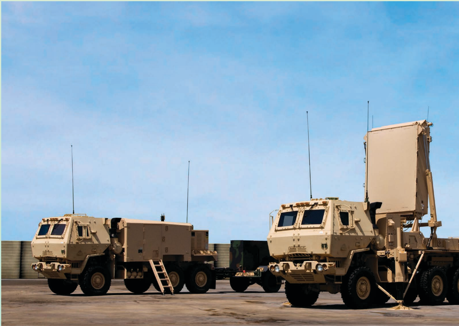
The AN/TPQ-53 system (shown here in its fully upgraded configuration) is the Army's next-generation counter-fire target acquisition radar. It is scheduled to replace the EQ-36 QRC in 2019. (Paul Salcel/Lockheed Martin Corp.)
