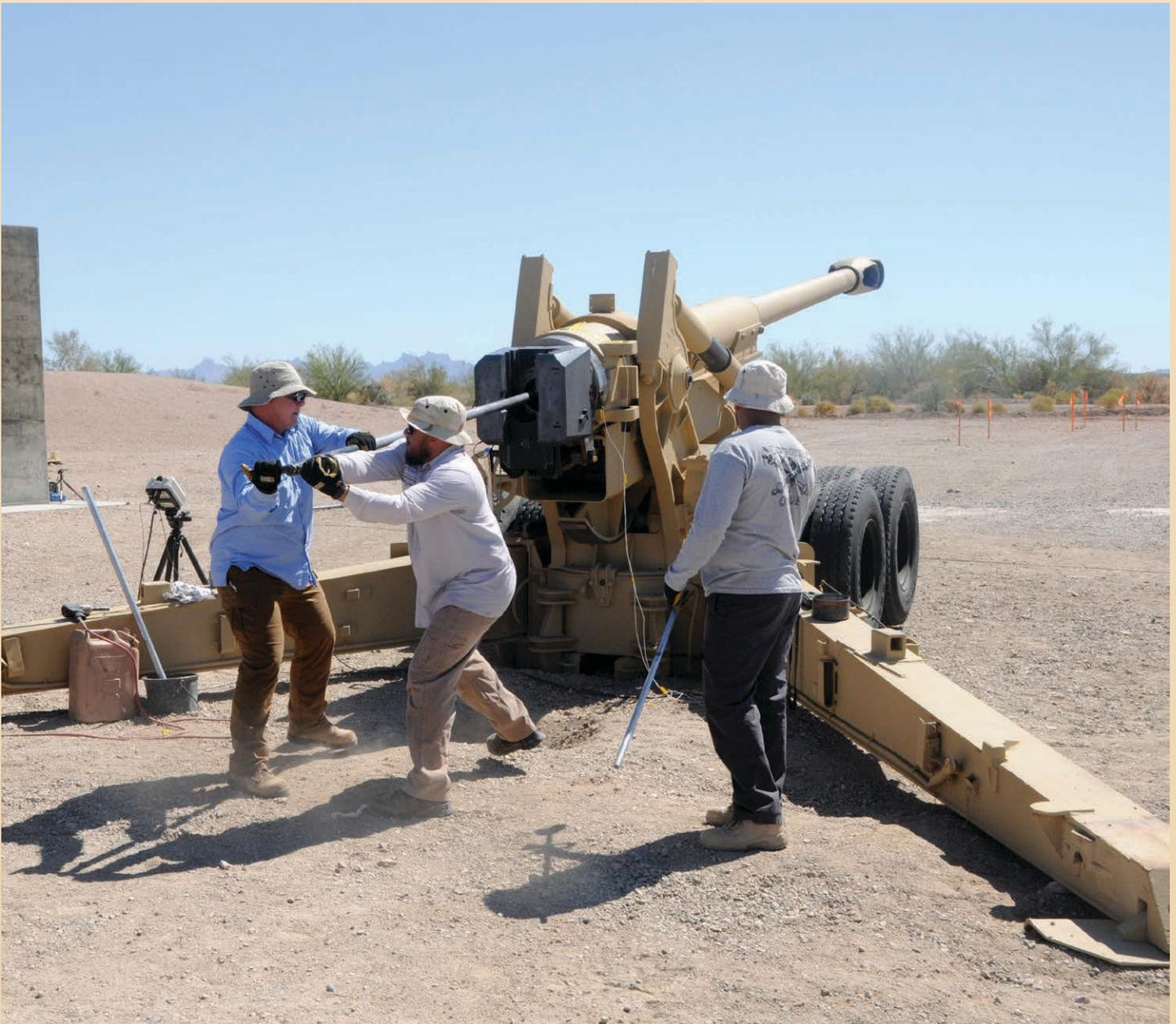
One critical component of the Extended Range Cannon Artillery program currently being tested at the proving ground is the XM1113 projectile, which exceeded 60 kilometers in a test conducted at U.S. Army Yuma Proving Ground in late May. The most significant difference is in the round's much larger rocket, which pushes out more than twice as much thrust as the legacy system. (Mark Schauer/U.S. Army)
